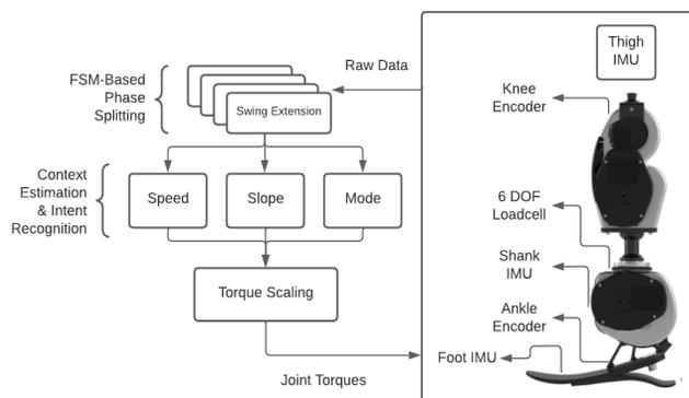
Figure 1. OSL sensors, control structure, intent recognition, and context estimation.
