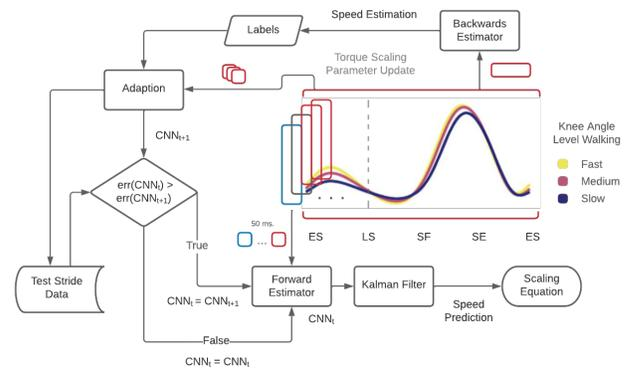
Figure 2. Adaptive pipeline schematic showing data flow to backwards estimator (evaluated every three strides) and forward predictor (evaluated every 50ms.).
