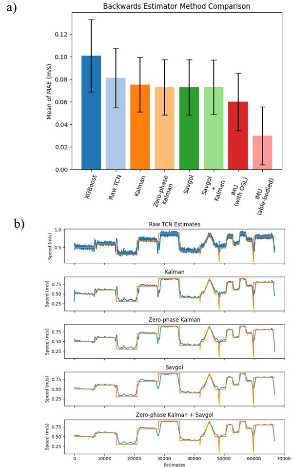
Figure 4. (a) Backwards estimator average MAE comparison. MAE = [0.101, 0.081, 0.075, 0.073, 0.074, 0.074, 0.060, 0.030], STD = [0.032, 0.026, 0.024, 0.024, 0.024, 0.024, 0.026, 0.026] m/s. (b) Filtered TCN estimations with different filters. The orange line is the ground truth values.
